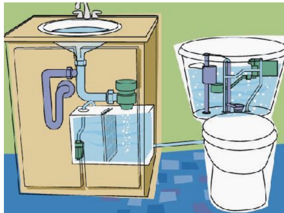
Figure 2: WaterSaver Aqus Greywater System (Australia)
